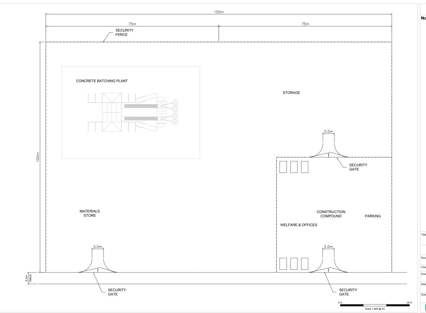
Note: This drawing is for illustrative purposes only Indicative Construction Compound Limekiln Wind Farm Section 36C Variation Source: Client: Infinergy Drawn by: Checked: Figure: 05/05/2021 4.4 Revision No: 1:500 @A3 **INFINERGY**
