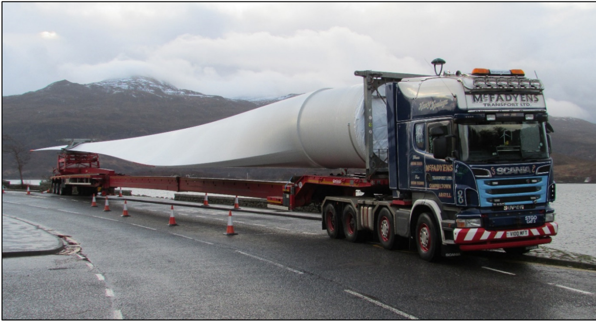
Figure 3 Typical Blade Transport using Super Wing Carrier
